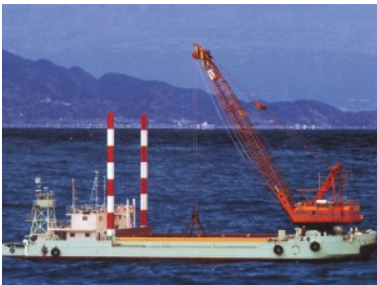
Ryuo: Multipurpose hoist ship with spud
